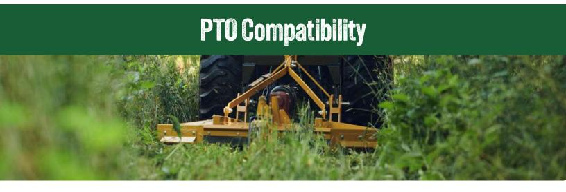
If the implement is powered by the tractor, such as a tiller or mower, you'll need to confirm it matches your tractor's Power Take-Off (PTO) specifications. Key details include:
